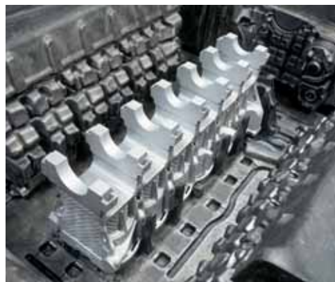
The R6 crankcase features a magnesium shell around an aluminum insert (image) that incorporates the cylinder liners and coolant ducts.
