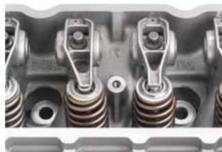
Unique hydraulic rollers for the LS7 help to actuate the larger valves and provide more valve lift.
