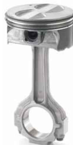
The LS7's aluminum flat-top pistons are connected to a forged-steel crankshaft with titanium connecting rods.
