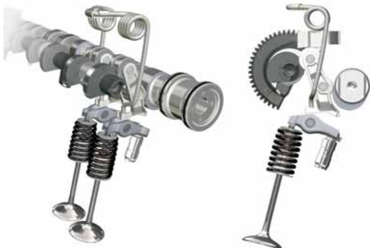
The R6 gets BMW's second-generation Valvetronic for higher engine speeds. The innovation adjusts valve opening times and valve timing infinitely according to accelerator pedal position and eliminates the need for throttle butterflies
