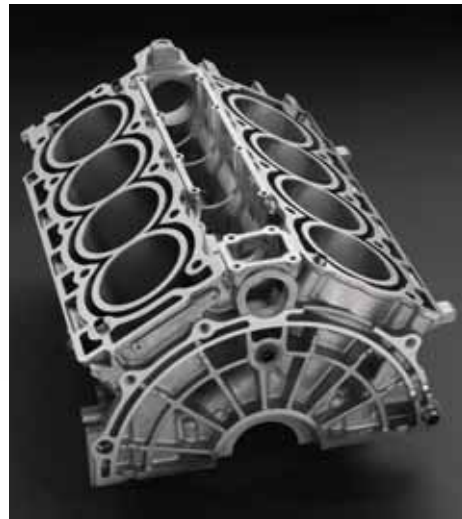
The 60° V8's narrow central valley leaves just enough space for the critical balance shaft in the location of an OHV V8's camshaft. The iron cylinder liners are cast into the high-pressure die-cast aluminum block.
