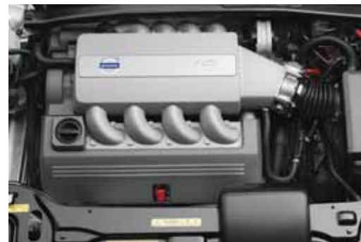
Volvo determined that only a very narrow 60° V8 would fit in the XC90's engine bay while preserving the requisite forward crumple zone.
