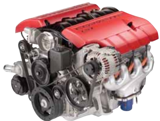
The 7.0-L LS7 for the 2006 Z06 produces 500 hp (373 kW) at 6200 rpm and 475 lb-ft (644 N-m) at 4800 rpm with the help of racing technology transfer.
