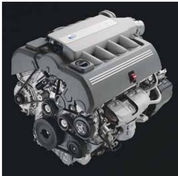
The compact 4.4-L Yamaha-built 60° aluminum V8 measures only 29.7 x 25 in (755 x 635 mm) and has a mass of 419 lb (190 kg), but produces 315 hp (235 kW).
