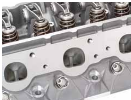
The LS7 cylinder heads are CNC-ported and have very large (by production-vehicle standards) intake and exhaust ports to speed airflow.
